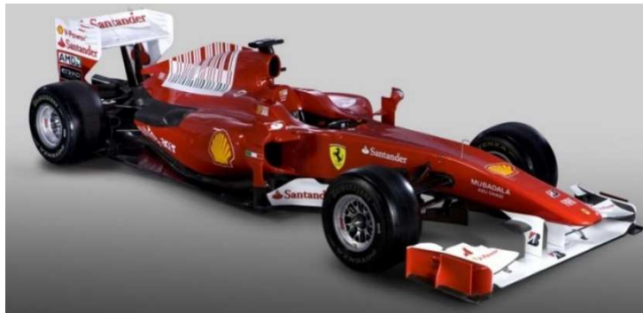
Figure 2 - Formula 1 car (2010), by Ferrari. Chassis and cockpits are currently manufactured by composite materials to ensure higher safety and lightness [5].
