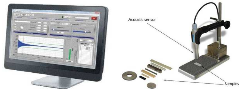
Figure 17 – Configuration of the Sonelastic solutions used to characterize the lamina in this study, highlighting the software and the basic support for small samples (SB-AP).
