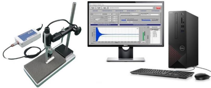
Figure 17 – Configuration of the Sonelastic® solutions used to characterize the lamina in this study, highlighting the software and the basic support for small specimens (SB-AP).
