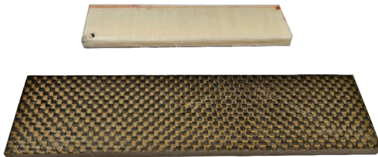
Figure 3 - Specimens of an ultra-high molecular weight polyethylene (UHMWPE) for ballistic armor and of an aeronautical monolithic panel made of carbon fiber reinforced plastic (CFRP). They are prepared for elastic moduli non-destructive characterization by Impulse Excitation Technique with Sonelastic® Systems [6].
