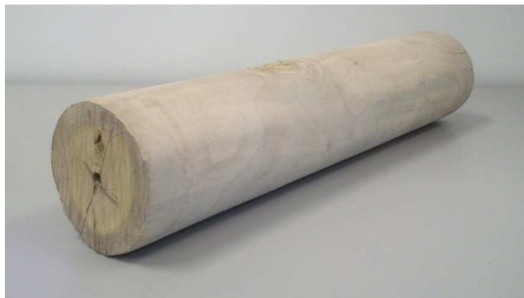
Figure 13 – Lathed wooden log with a good superficial finishing, highlighting the central region of the log composed by heartwood, and the external region, composed by sapwood.
