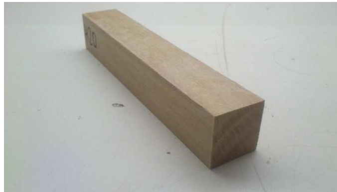
Figure 8 - Sample presenting fibers aligned parallel to its length.
