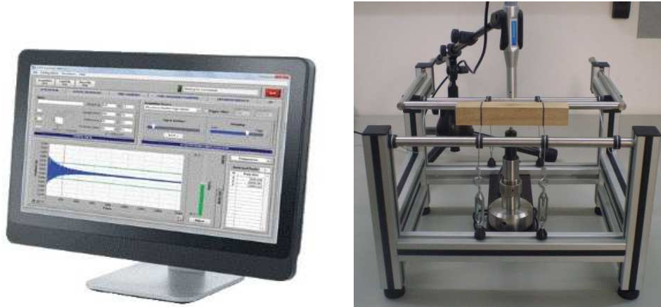
Figure 10 - Sonelastic® equipment developed by ATCP Physical Engineering for elastic moduli characterization via Impulse Excitation Technique.
