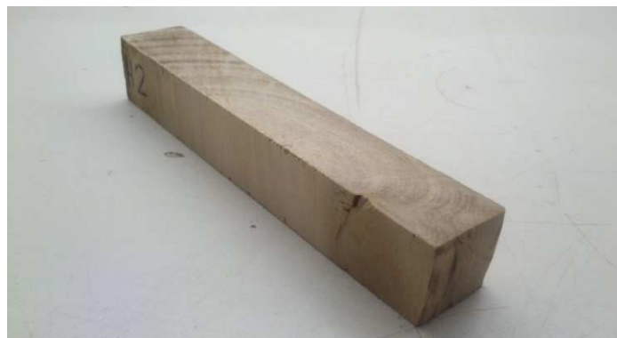
Figure 9 - Sample presenting combined radial and tangential orientation parallel to its length.
